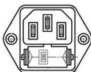
Fuse holder with clamping lugs
